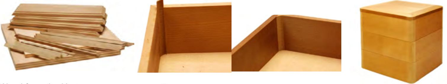
Wood from the Ho tree (Magnolia family) and top-quality Shina plywood is evaluated and ried thoroughly. The parts to be used in the final product are cut out and planed.
